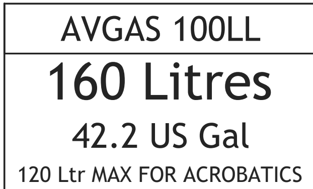
Adjacent to refuelling receptacle
